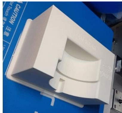
b) 3D printed, Brushless support
